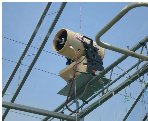
Figure 31. Mechanical fogger. Source: Damm Corporation. Photo: Louis Damm,
