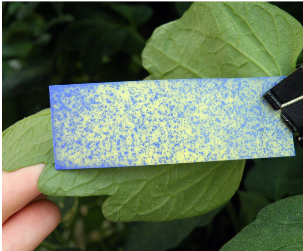
Figure 27. Under-leaf coverage with a manually towed sprayer using TeeJet VisiFlo hollow cones (TX-VK3) operating at >300 psi.
